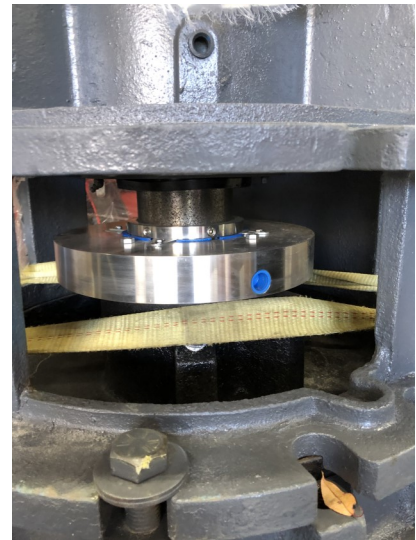
SH pump with new style seal
